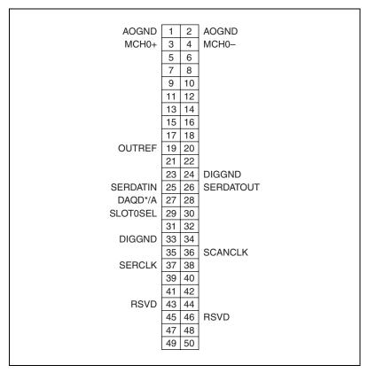
Figure 1. SCXI-1100 Rear Connector Pin Assignments
